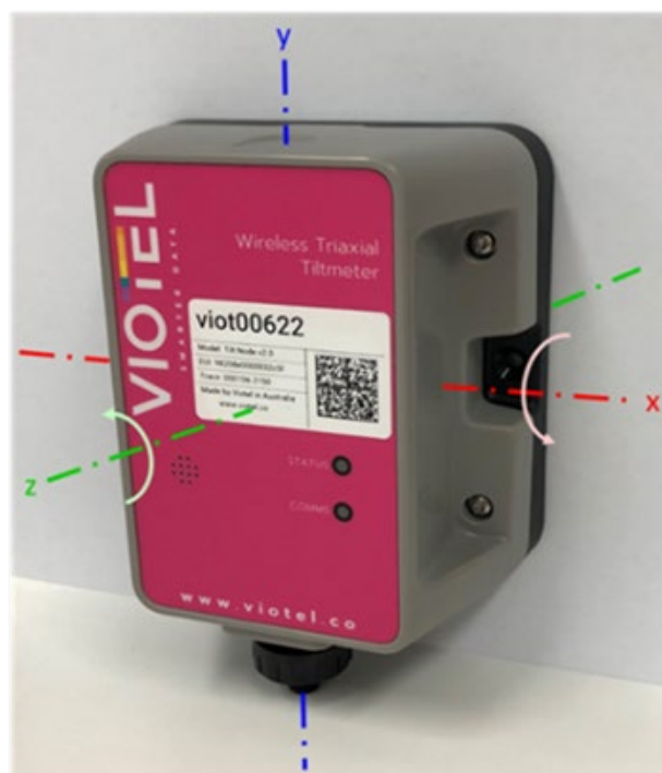
Figure 5 Photo showing X, Y, Z Axis Orientation
