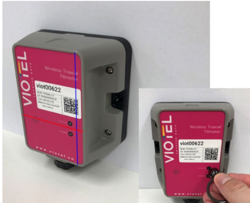
Figure 4 Photo highlighting location of the Magnet
